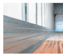
■ Sidewall Protection from fork lift and cargo damage is provided by a 10.25" high corrugated galvanized, roll-formed steel scuffband that extends full length to the front wall. Additional methods of sidewall protection vary in types, materials, and heights.
