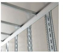
**Roof System** features tension-mounted aluminum roof sheets permanently bonded to galvanized, anti-snag roof bows, and then secured with two fasteners to the side rails for reinforcement.
