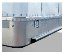
Front End Protection from impact and corrosion is provided by a stainless steel front bottom rail and stainless fasteners. An optional weld-on stainless steel roll lip protects the upper coupler from fifth-wheel impact.
