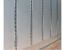
**■** Posts and Spacing **Options** include galvanized steel hat and shallow logistic posts for more interior width and blocking or decking capability. Closer upright spacing is available in 12", 16", and 24" centers for heavy-duty operations.
