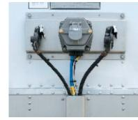
are mounted to the front wall on an aluminum mounting channel for easy access and reduced maintenance. A large air and electrical protector allows for easy access to lines.
