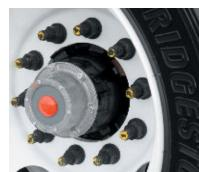
Painted Black Hubs & Powder-Coated Wheels improve appearance over the life of the trailer. Powder-coated wheels provide enhanced corrosion protection and durability, while reducing maintenance and refurbishing frequency.
