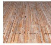
■ Durable Floor System provides strength in key high stress areas. A net 1.38" laminated hardwood floor is secured with 2 screws in an alternating pattern, and is available with 3 screws for added strength.
