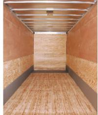
■ Hardwood Plywood Lining Horizontally installed with wafer-head metal drill screws for a snag-free lining. Steel hat section uprights are located on 24" centers with extra uprights in high stress areas.
