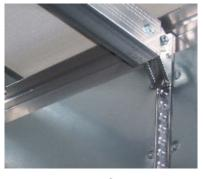
■ Double Decking Option The Double Dex option creates a second deck to accommodate additional cargo by using captive beams with a recessed track.
