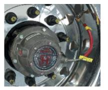
Automatic Tire Inflation Systems help extend tire life and increase fuel efficiency by using compressed air from the tractor to maintain tire pressure settings during operation. Multiple tire inflation systems are available as options.
