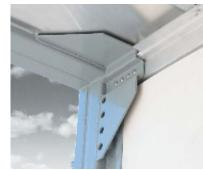
■ Rear Frame Reinforcement **Gussets** minimize racking and ensure that the frame remains square throughout the life of the trailer utilizing 0.25" steel to reinforce the rear header to top rail connection, maintaining a 110" inside height the full length of trailer.
